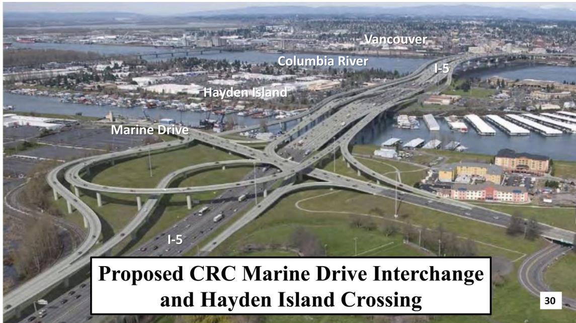
Here is the proposed 2012 design for the same interchange and river crossing. Note the increased complexity and increased heights of the bridges, blocking much of the view near the river edges and on Hayden Island. This is not a new bridge; it is a major freeway expansion project, that just happens to cross a river.
